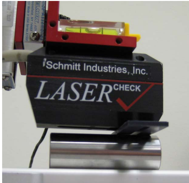
Lasercheck Sensor Lowered to pre-set 0.1 inch gap using stand-off plate
